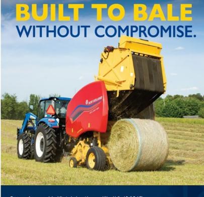
Get top performance and durability in dry hay with a rugged New Holland Roll-Belt™ 450 or 460 Hay Special round baler. The 71-inch-wide pickup carefully gathers all your hay as the ActiveSweep™ feeding system relentlessly moves it from the pickup into the chamber. That's where perfect square-shouldered bales are built consistently with the proven combination of steel rolls and Mini-Rough-Top laced belts. Get no-frills baling without compromising performance.
